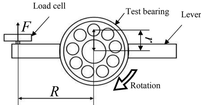
Fig. 3 Schematic illustration of friction coefficient measurement method.
