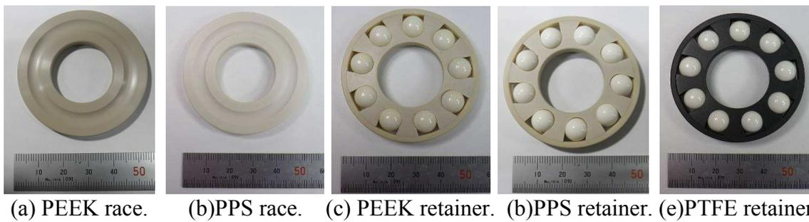
Fig. 1 Bearing sample elements.
