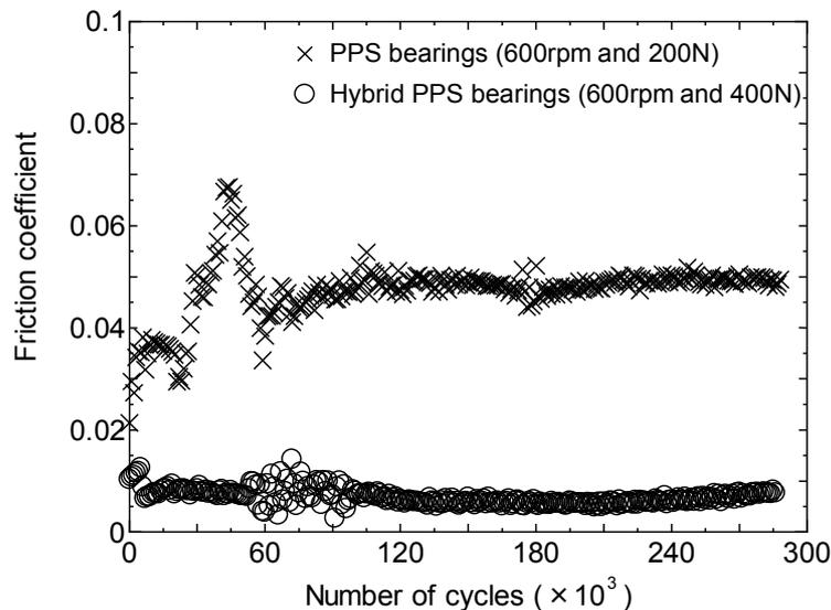
Fig. 4 Relationship between number of cycles and friction coefficient in PPS-races.
