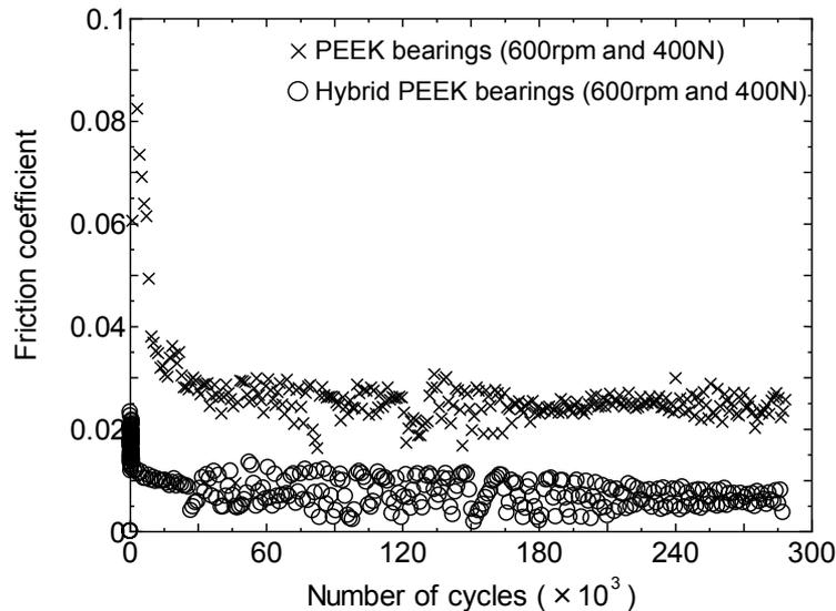
Fig. 5 Relationship between number of cycles and friction coefficient in PEEK-races.
